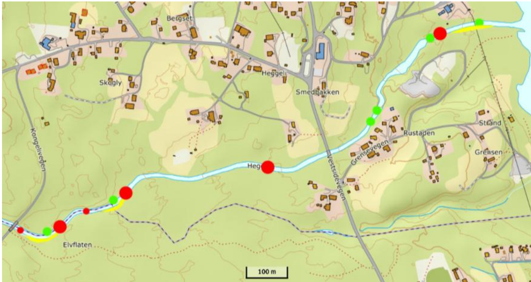
Figure 4. Measures proposed by Colman et al., 2019. Yellow areas indicate the proposed modifying of the riverbank. Green circles indicate the proposed excavation and stone reinforcement of pools. Red circles indicate proposed locations for spawning gravel placement. The size of the red circle (large/small) indicates the amount (high/low) of spawning gravel. Map base: Kartverket 2019 (WMS). Source: Colman et al., 2019.
