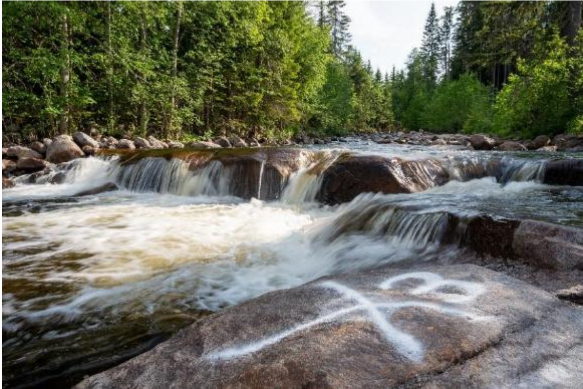
Figure 5. Ground control point near a rapid, marked with environmentally friendly chalk spray.
